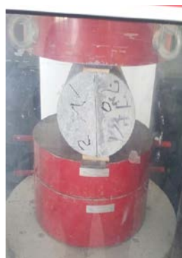
Figure 4: Splitting tensile test set-up.
