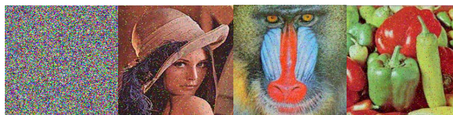
Figure 5: Data loss. (a) The encrypted images with data loss; (b) the decrypted Lena image with different data loss; (c) the decrypted Mandrill image with different data loss; (d) the decrypted Pepper image with different data loss.
