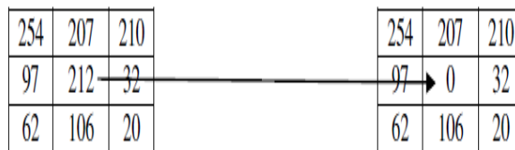
Figure 1: The central pixel value is corrupted by Pepper noise
