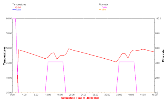
Figure 7.b: The relationship between the temperature of the drawn water and the flow rate and the simulation time, which is two full days
