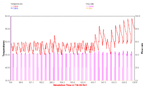
Figure 7.a: The relationship between the temperature of the withdrawn water and the drag rate and the time that represents a full month and the draw were in the evening, ie before sunset
